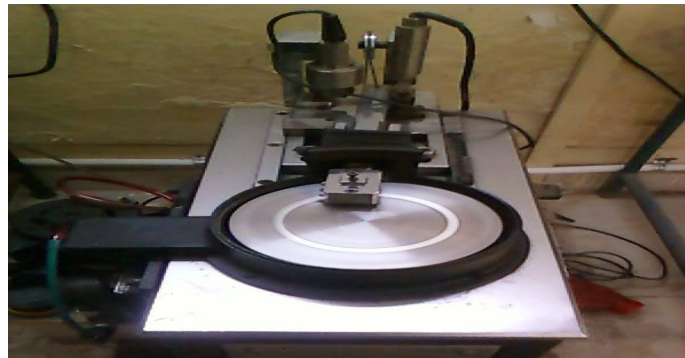
Fig 1: Pin on Disc machine [Courtesy: MNIT, Jaipur]
