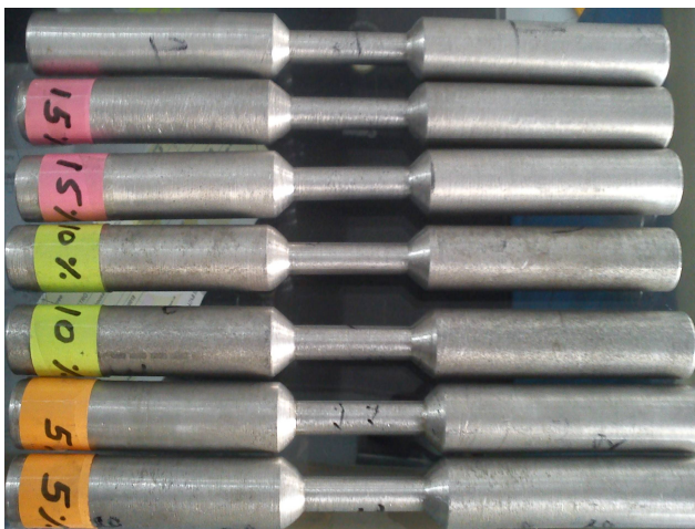
Fig. 3: Cylindrical pins used for wear test
